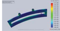
Figure 6: Stress Applied on Rail
